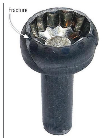
Fig. 4 Fracture on cold-forged bolt
