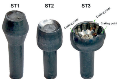
Fig 3. Cracks on the head
