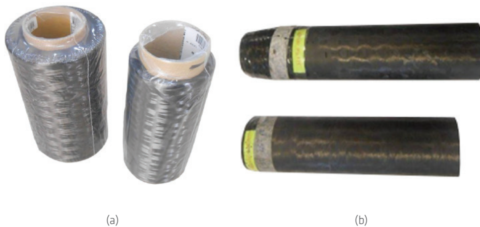
Figure 4. UMS 40-IMS 65 carbon fiber rolls (a) and composite tubes with fiber orientation of [90/\pm 45/\pm 15/90]_n (b).
