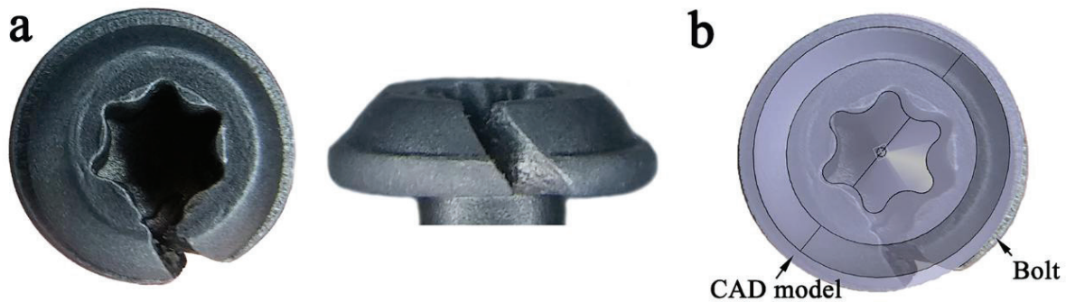
Figure 3. Crack evolution on the bolt; (a) top and front view and (b) comparison of the damaged bolt and CAD model.
