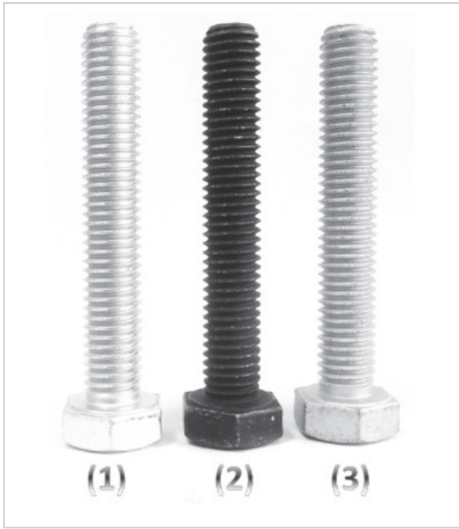
Şekil 1: Bolt specimens coated with 1-) Zn Cr+3 + TnT 11, 2-) Delta-Protekt® KL100 + Delta Seal GZ Black and 3-) Delta-Protekt® KL100 + VH301 GZ
